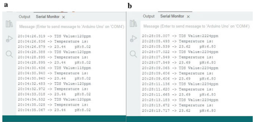
Fig. 7 a, b Readings before and after adding nutrients and pH balancing solution to the reservoir water tank which contains tap water with pH-8 and TDS 120 ppm
