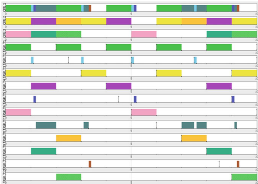
Fig. 6 Gantt chart for 11 tasks with 3 CPUs U_{RM} schedulability test-based algorithm
